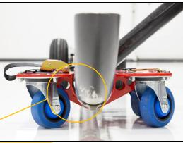
Retainer to keep skid safely aligned
