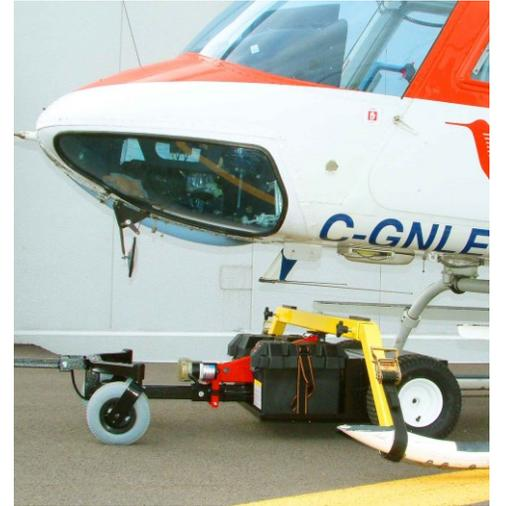
**Quick connect Jack head** on V201 allows for instant attachment exchange from one to the other (AT44 to AT45)
